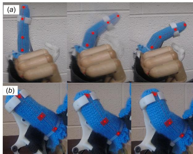
Fig. 10 Experimental analysis at various stages of the bending motion: (a) index finger and (b) thumb
