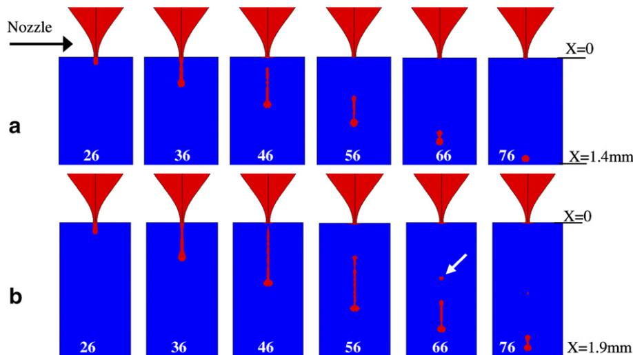
Fig. 7. Simulation results for duty cycle of 1% at: (a) 350 mbar; (b) 500 mbar.
