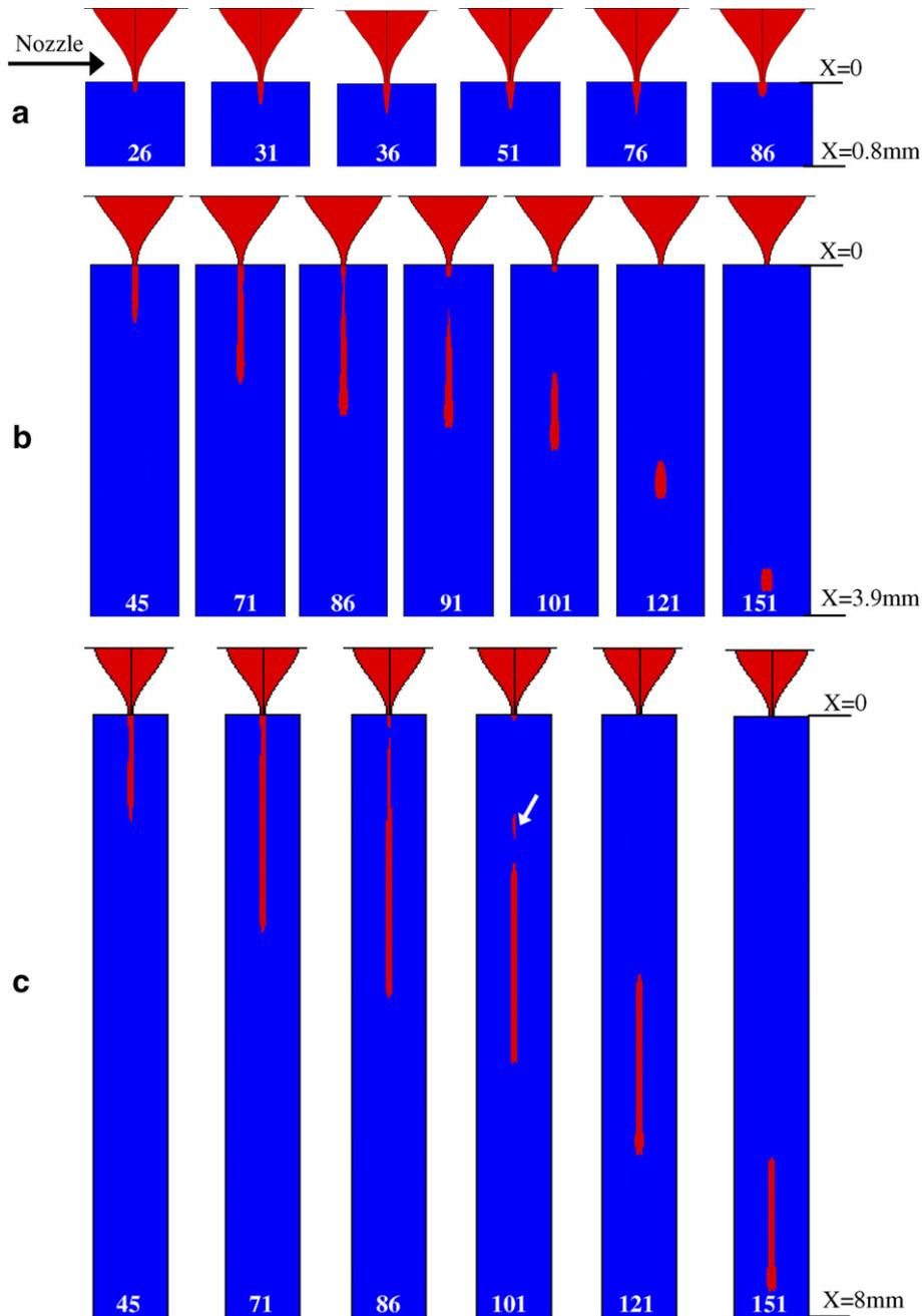
Fig. 6. Simulation results for duty cycle of 5% at: (a) 200 mbar; (b) 350 mbar; (c) 900 mbar.
