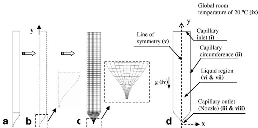
Fig. 3. Model geometry, finite element mesh and boundary conditions.
