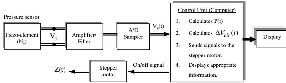
Fig. 2. Real-time closed loop pressure control.
