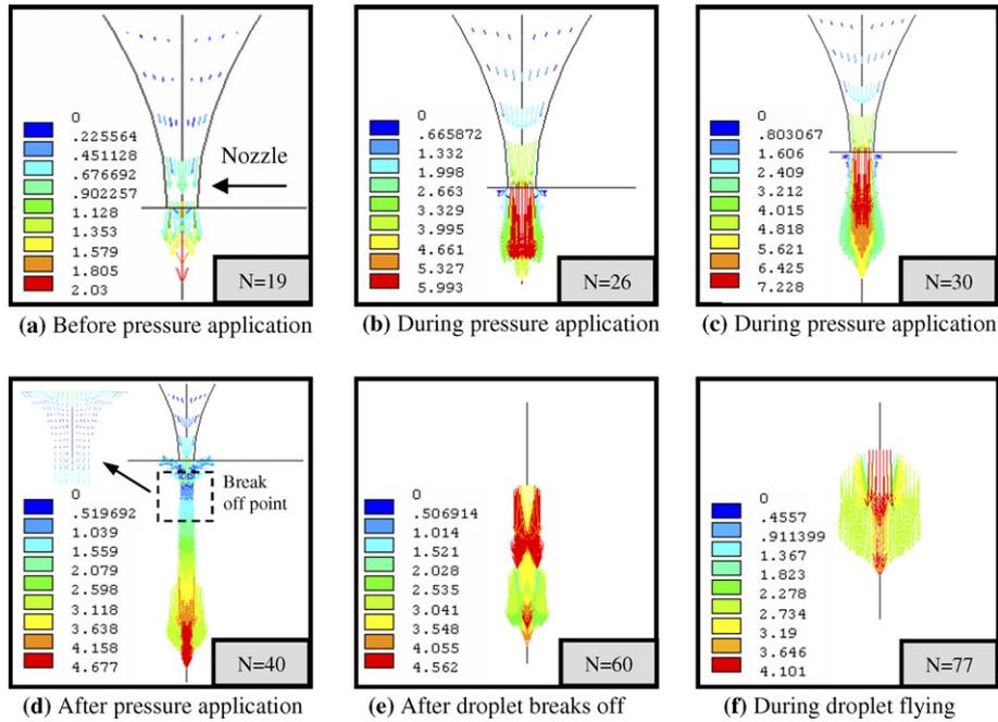
Fig. 9. Velocity vector analysis at different time samples.
