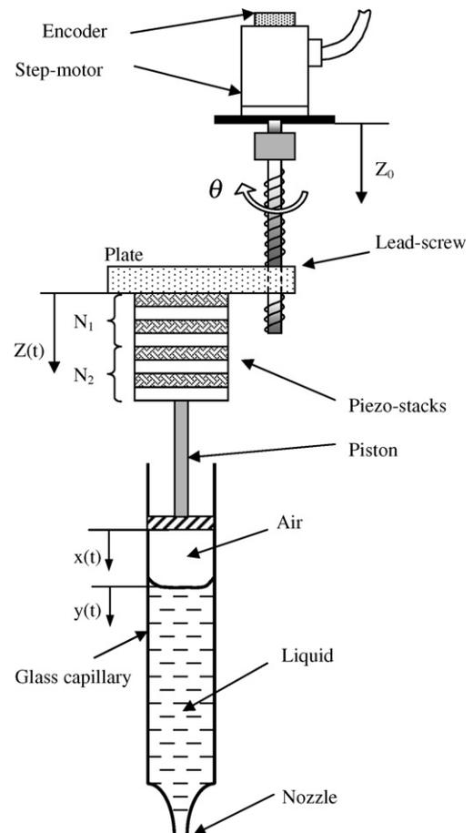
Fig. 1. Schematic of a piezo-driven-piston dispensing system.
