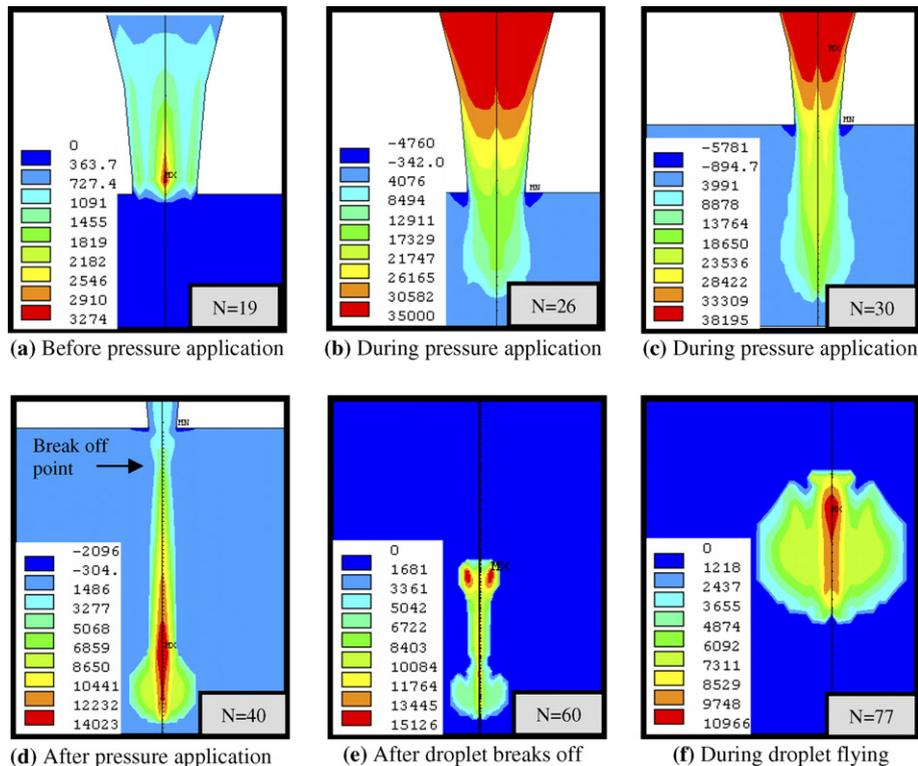
Fig. 10. Pressure distribution analysis at different time samples.
