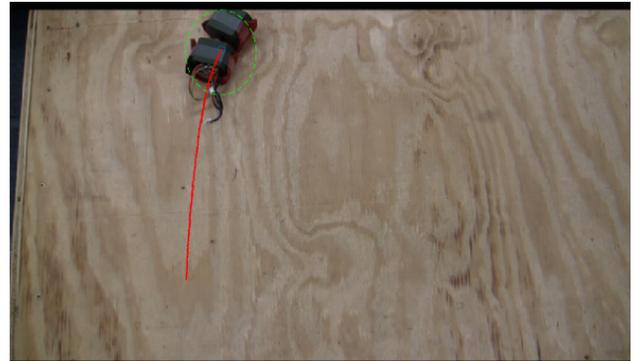
**Figure 7. Steering of MMIR on wood.**
