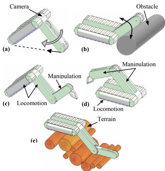
Fig. 2 (a),(b) sample mobility configurations; (c),(d) sample manipulation configurations; (e) configurations for enhanced traction.
