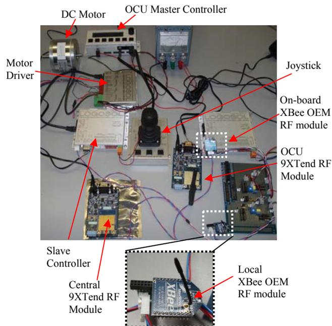
Fig. 7 Experimental setup for RF comm. testing.
