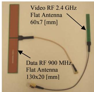
Fig.4 Embeddable flat antennas for video and data RF communication.
