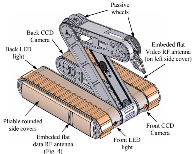
Fig. 3 Fully loaded mobile manipulator.
