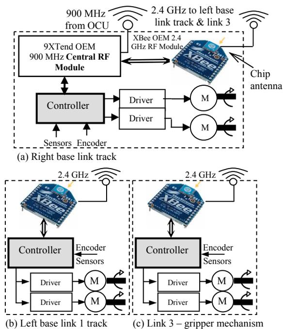
Fig. 6 Hardware architecture: (a) right base link track; (b) left base link track; (c) link 3 – gripper mechanism.
