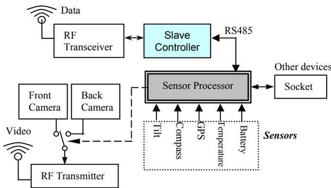
Fig. 8 Sensors and cameras layout.
