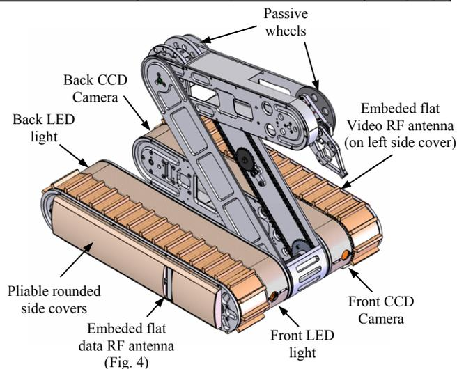
Fig. 3 Fully loaded mobile manipulator.
