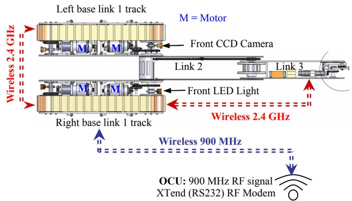
Fig. 5 RF communication layout.
