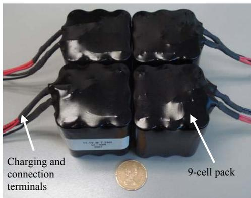
Fig. 9 Li-Ion battery packs assembly.
