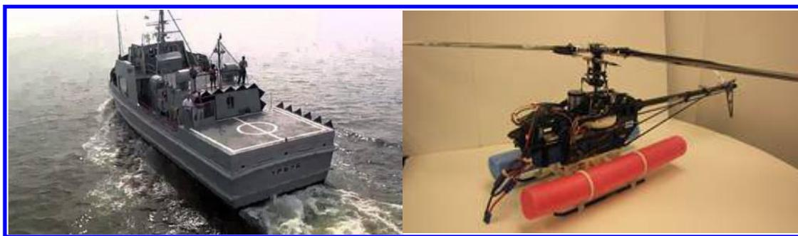
**Figure 1a. Modified YP676 naval training vessel with flight deck (left); b). RC helicopter with retrofitted instrumentation board and flotation system (right).**
