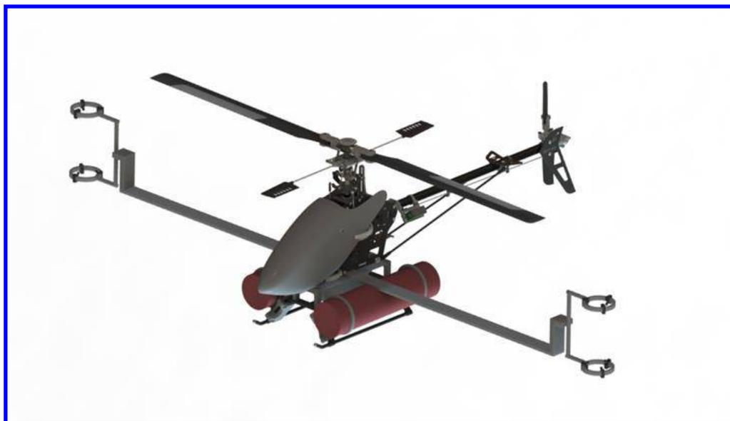
**Figure 6. Proposed TREX 600 helicopter with anemometers for direct measurement of air wakes.**
